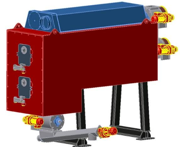
Through the sector gate, the raw material reaches the converter screw, which then transports the biomass through a combustion chamber. Within this chamber, the biomass is dried, pre-heated and pyrolysed, and further energy is added in the reformer chute. As during the production of active carbon, a very hot gas mixture passes through the smouldering biomass. The residence time is extremely long and leads to an exceptionally clean biochar..
